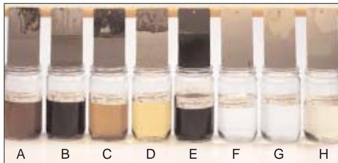
*Note the difference in appearance of these mild steel panels immersed for 28 days in adjuvants. The panels placed in All-Purpose Spray Adjuvant (G), and in APSA-80 (H) are corrosion free. Panels A, B, C, D, E, and F were placed in competitive brands.*
